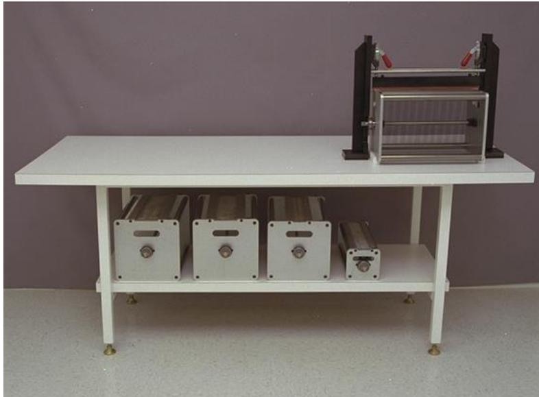
After the adhesive has cured, the suture rack is placed into the suture-cutting fixture as shown. The sutures are held in position and are cut from the rack using a hand held rotary knife. The sutures are cut through the center of the two-inch tipped portion leaving a one inch tipped length on the end each suture.
